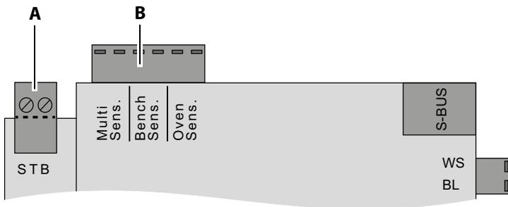
**A** Terminal plug for safety temperature limiter
