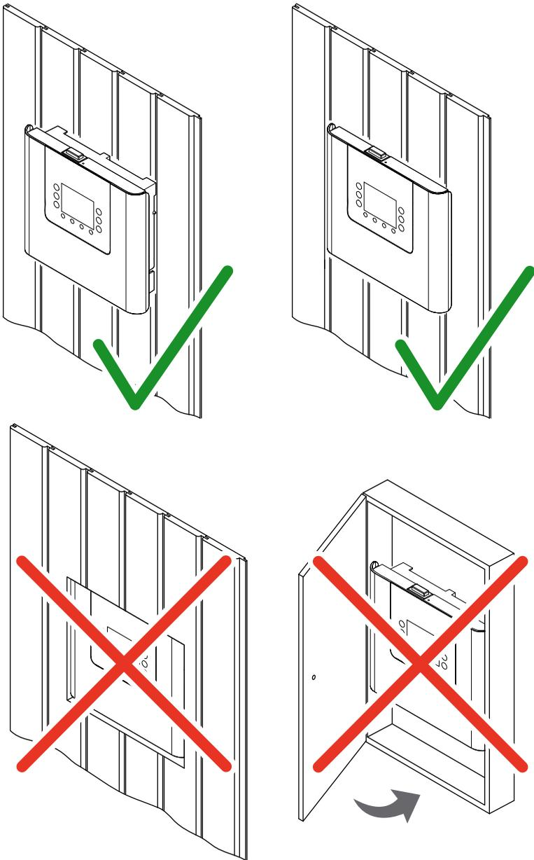
☒ Proper and improper mounting of the control unit
