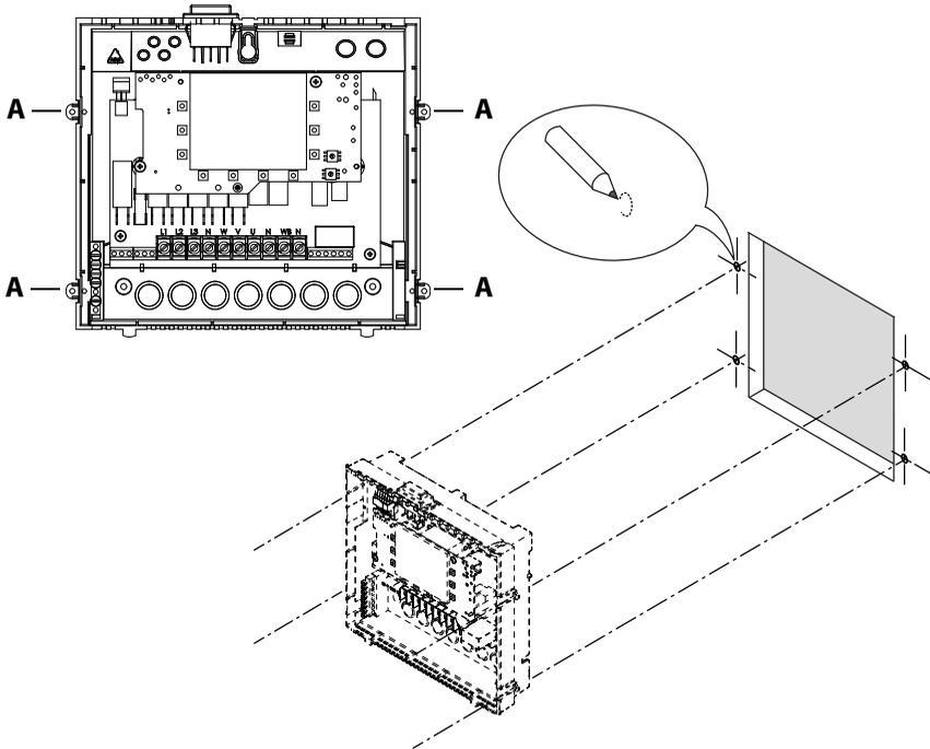
**A** Tabs with mounting holes for screws
