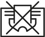
Objects left on the heater and/or directly in front of an IR emitter can catch fire and lead to fires.
